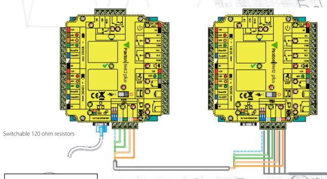
The Net2 plus plugs directly into the TCP/IP Ethernet network via a standard RJ45 connection box
